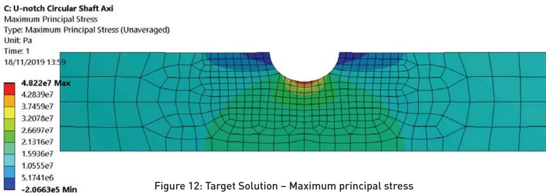
Figure 12: Target Solution – Maximum principal stress
