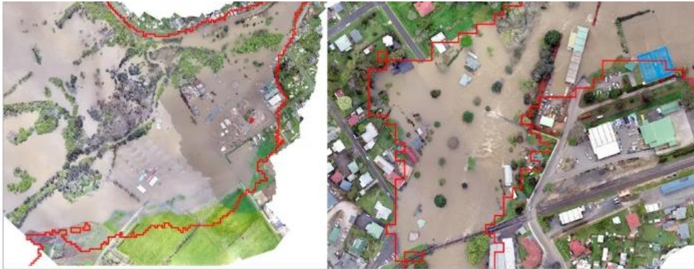
A comparison of the InfoWorks ICM peak extent output using forecast rainfall and drone images against the actual peak for the major flood at Deloraine in October 2022.
